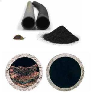
Comparison of carbon build-up in a strand annealing furnace, NiCr tube(left) and APMT(right).
