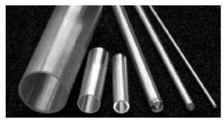
components deteriorate much faster. Unlike ceramic casings, sapphire structure is perfectly homogenous throughout the whole product. Perfect crystal lattice also prevents the surface of sapphire tubes from outgassing.
