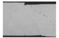
Micrograph of standard Pt wire after 6 hours at 1400 °C under a tensile stress of 2.76 Mpa, showing a large grain structure and resulting grain boundary movement.
