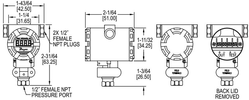
The **Series IWP Industrial Weatherproof Pressure Transmitter** provides an exceptional value solution to pressure measurement in industrial conditions requiring high-performance, stability and long service life. The precise operation under dirty and wet conditions, make the Series IWP an ideal choice for petroleum, chemical and metallurgical industry applications.
